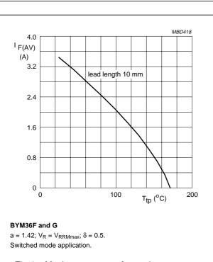
Fig.4 Maximum average forward current as a function of tie-point temperature (including losses due to reverse leakage).
