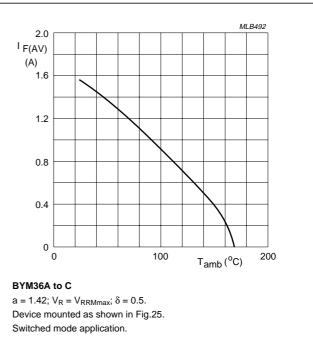
Fig.5 Maximum average forward current as a function of ambient temperature (including losses due to reverse leakage).
